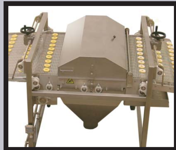
Removing Flour From Product With the Flour Removal Conveyor
