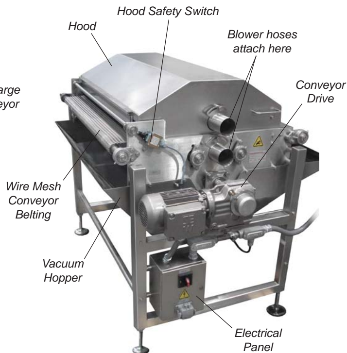
Flour Removal Conveyor (using a blower)
